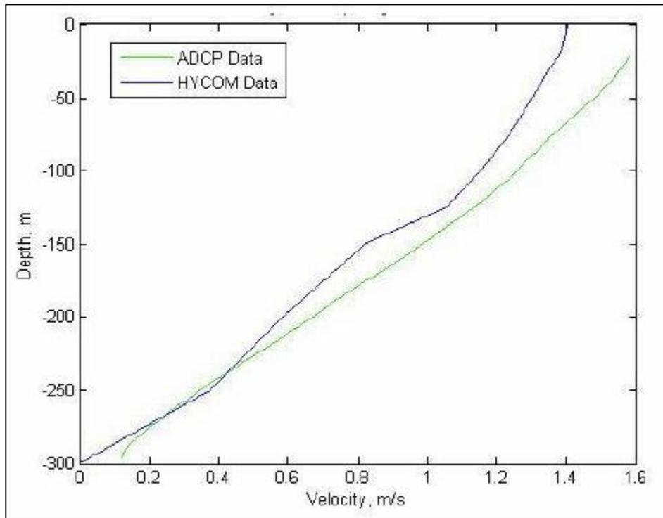
**Figure 3:** Comparison of 13-Month Averages of Northward Velocities from HYCOM and The SNMREC ADCP.
