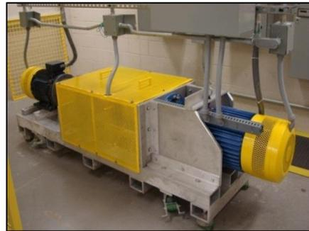
20kw Dynamometer for Generator Testing
